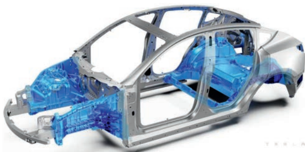
Figure 1.29 Two Cast Body Pieces Highlighted Photo: Tesla - Model Y Body Structure
